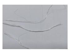
Steel Wire Glass Fiber Cloth has all the advantages of ordinary glass fiber cloth, and also has its unique excellent properties of high strength, low shrinkage and no deformation. The strengthening with the food grade S.S wire significantly improves the tensile power. Weave can be one-directional (stainless is only inserted in warp yarn) or two-directional (stainless is inserted in both warp yarn and weft yarn)
