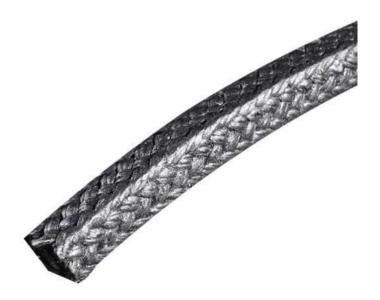
Carbonized fiber packing braided from shrink-proof synthetic fiber impregnated with PTFE, Silicone-oil-free. Oxidized fiber has high strength and good thermal conductivity, PTFE makes the packing have excellent self-lubrication.
