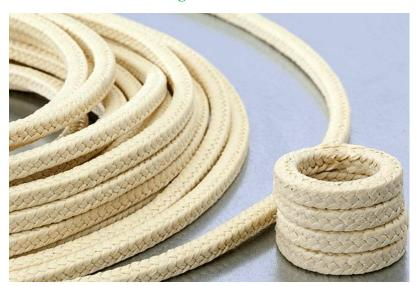
Aramid fiber packing braided from high quality aramid and kevlar fiber with PTFE impregnated and lubricant additive. It is wear resistant but may damage the shaft is not used properly. A minimum shaft hardness of 60HRC is therefore recommended.
