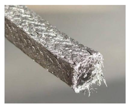
Super Graphite Packing specially for high pressure valves, braided from expanded graphite yarns with corrosion inhibitor, reinforced with inconel wire. Each yarn is round braided with inconel mesh outside again. The mesh is jacketed.
