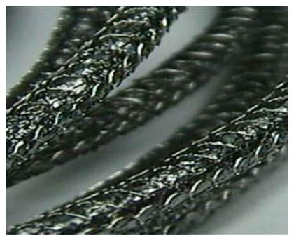
Jacketed Graphite Packing braided from graphite yarns with metal alloy and glass fiber casing like the socks outside. Used in any steam valves applications.
