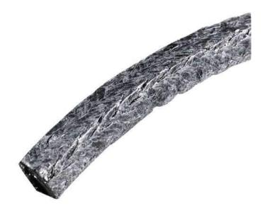
Graphite Packing with PTFE Impregnated is braided from Expanded graphite yarns which impregnated with PTFE as a blocking agent thus creating a non-straining packing. The yarns are reinforced by textile fibers.
