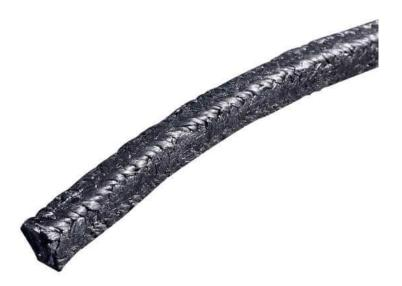
Graphite packing with carbon fiber corners is a multi-fiber packing, braided from expanded graphite yarns and carbon fibers, the diagonally braided from graphite yarn, reinforced in all four corners with carbon fibers. The corners and body make the packing three times more resistant to extrusion and increase the pressure handing capabilities compared to traditional graphite packings.
