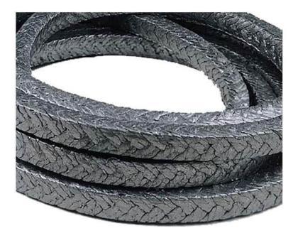
Flexible graphite packing are braided from flexible graphite yarns, which are reinforced by cotton fiber, glass fiber, carbon fiber, etc. It has a very low friction, good thermal and chemical resistance and high elasticity.
