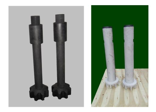
During aluminum and aluminum alloy smelting, hydrogen produced by chemical action with steam diffuse in molten aluminum, which will cause inner structural defect to aluminum products. In order to avoid such defect, most aluminum plants apply dissolved gas floating method to purify molten aluminum. i.e. inert gases such as nitrogen, argon is injected into molten aluminum, and hydrogen will be brought to molten aluminum surface with spread and rise of inert gas.
