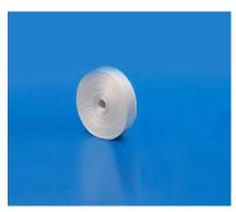
Fiberglass (or glass fibre) woven tapes are fabricated from high quality type E fiberglass that will not burn and will withstand continuous exposure to temperatures of  $1,000^{\circ}$ F /  $538^{\circ}$ C, and it features excellent electrical insulation.
