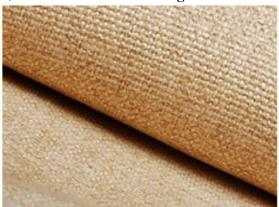
Higher strength than untreated fiberglass with superior insulation properties, vermiculite coating disperses heat along surface of the material preventing transmission of heat through the fabric. Excellent resistance to abrasion and molten metal and sparks than standard fiberglass cloth. Continuous service to  $1,500^{\circ}F$ , intermittent to  $2,000^{\circ}F$ . Heavy duty welding blankets and curtains, stress relief blankets.
