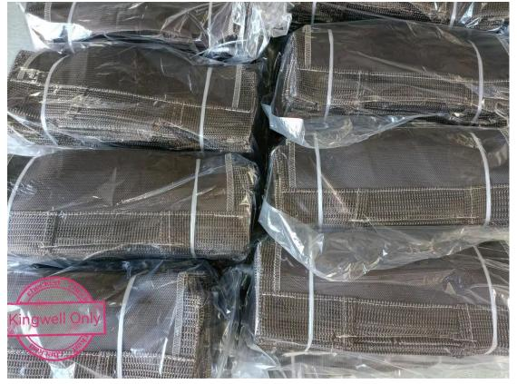
Which are specially designed and woven for the diffusion and filtration of aluminium. High twist yarns are used to control strand diameters and resist flattening or distortion under pressure from contact with molten aluminium.
