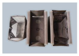
When molten aluminium is introduced by the Combo bag, there will be almost no Fire or Smoke.
