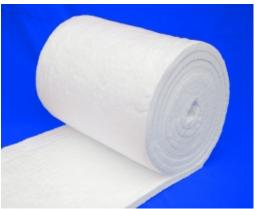
**Kingwell** Ceramic Fiber Blanket is made of special ceramic long-fiber that is produced by the melting of very pure raw materials in double surface meeding process without binders and with good stability in a large range of temperature. The process of double surface needling increase interweaving and tensile strength.
