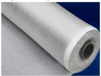
Woven roving is a fabric made by interweaving roving. This weave has an excellent dimensional stability. It can be compatible with many resins such as polyester, epoxy resins and vinyl ester, and is mainly used for hand lay-up of large, high-strength FRP products such as boats, automobile parts, storage tanks, furniture and other FRP products.
